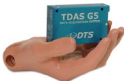
TDAS G5 DAS 32 Channels Size: 25 x 54 x 85 mm
